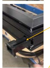
After removing the mushroom bolt holder, you need access to the lock. To do this, gently tap out the 'shot bolt panel guide' to reach the top shoot bolt, this will need to be done at the bottom of the panel also. Once exposed, you can remove the lock completely.
