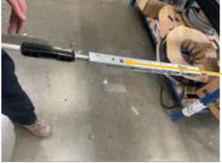
Once the shoot bolt guides are removed from both the top and bottom of the panel, you can pull out the entire lock, including the part that needs to be replaced, whether it's the top lock, bottom lock, or both.
