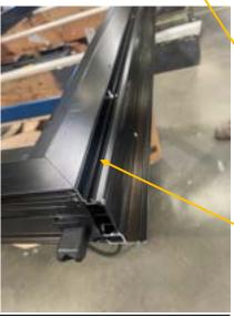
Once the mushroom bolt and screws have been removed, take out the 'closing rebate gasket' to expose the screws for the rebate.
