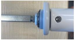
A sacrificial cut spindle is required for internal/external lever handles. This design enhances security by allowing the spindle to snap at the week point, under force or attempted break-in. The drill holes accommodate the grub screws used in MK3 lever handles. See the photo for reference.
