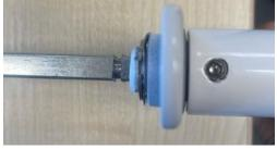
A sacrificial cut spindle is required for internal/external lever handles. This design enhances security by allowing the spindle to snap at the weak point, under force or attempted break-in. The drill holes accommodate the grub screws used in MK3 lever handles. See the photo for reference.
